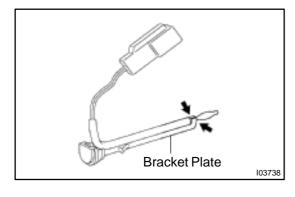
(c) Release the 2 claws and remove the thermistor from the bracket plate.
